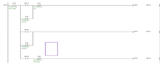
Gambar 19. Ladder Menonaktifkan Internal Relay
