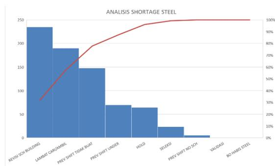
**Gambar 6.** Diagram pareto chart analisis shortage material steel belt
