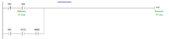
Gambar 22. Ladder PLC Servicer IP
