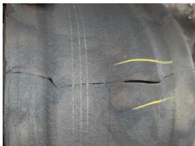
Gambar 27. Gambar defect tread open splice
