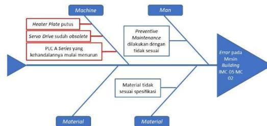
Gambar II. *Fishbone Diagram* Permasalahan Mesin *Building* BTU
