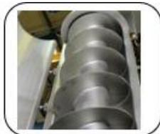
Gambar 17. Horizontal Screw Conveyor
