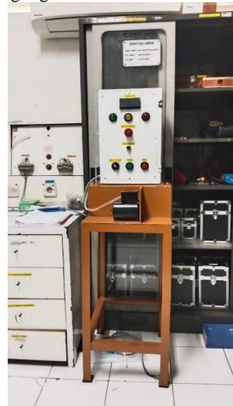
Gambar 12. Alat media kalibrasi tachometer
